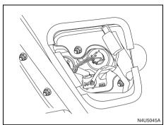
To replace a backup lamp or a tail/stop lamp bulb:
